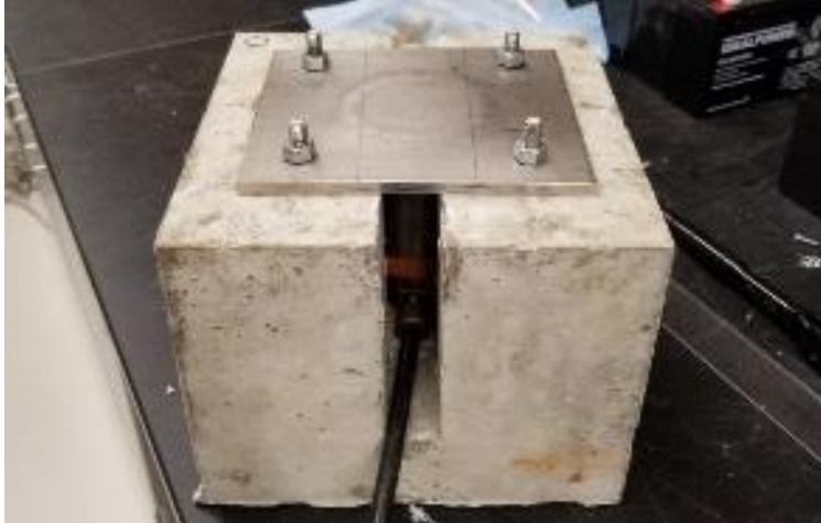
Figure 19. Impact plate mounted to concrete block. View of electrical wire conduit routed through inner channel.
