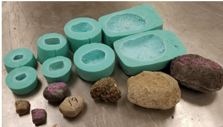
Figure 31. Particle tracking synthetic tracer stones, stone molds, and original stones.
