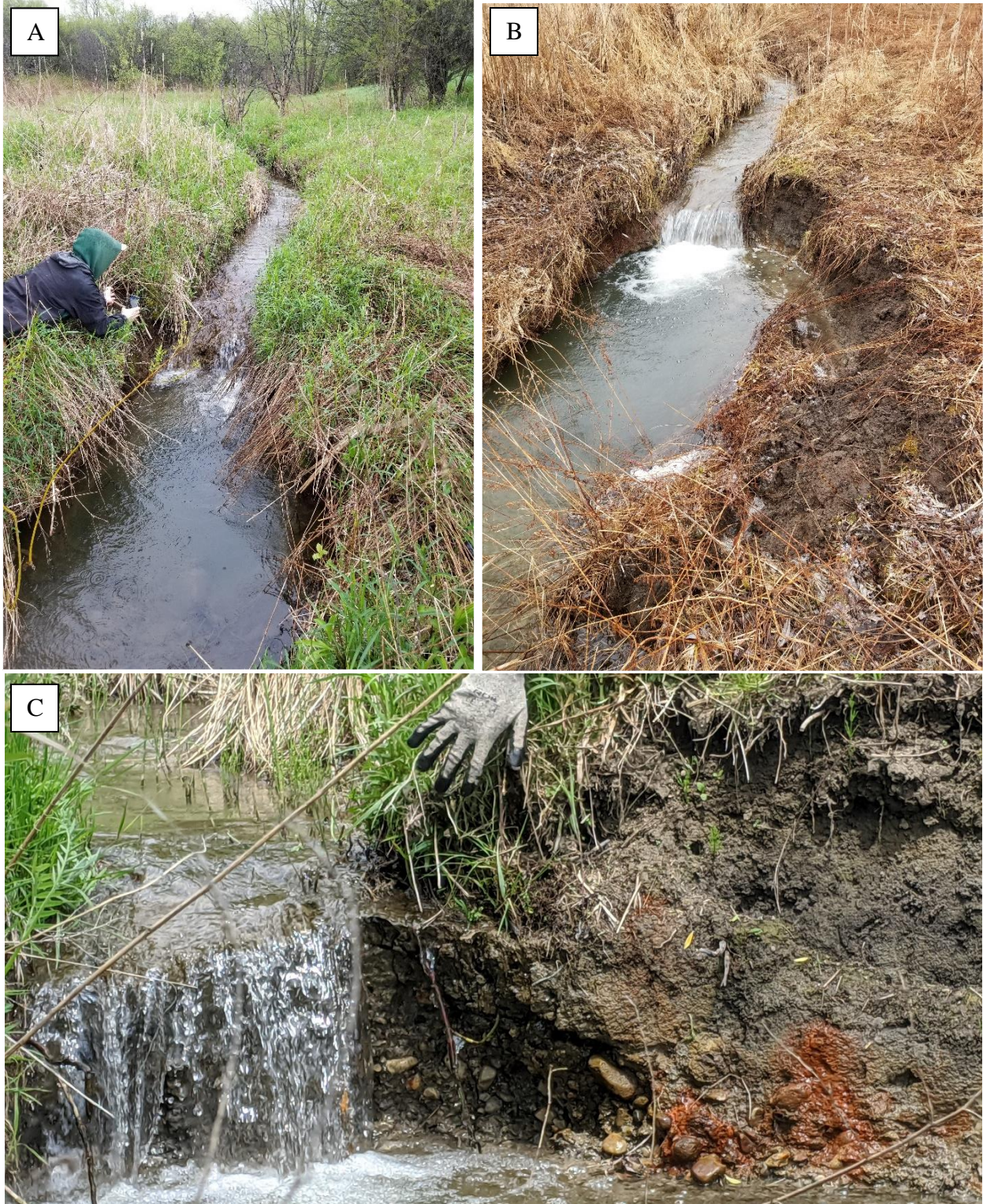
Figure 39. Visual comparison of headcut over study duration. (A) Headcut location on May 23, 2019. (B) Significant advancement first observed on March 17, 2020. (C) View of gravel particles embedded within till on June 1, 2020 (Photo credit: Bruce MacVicar).
