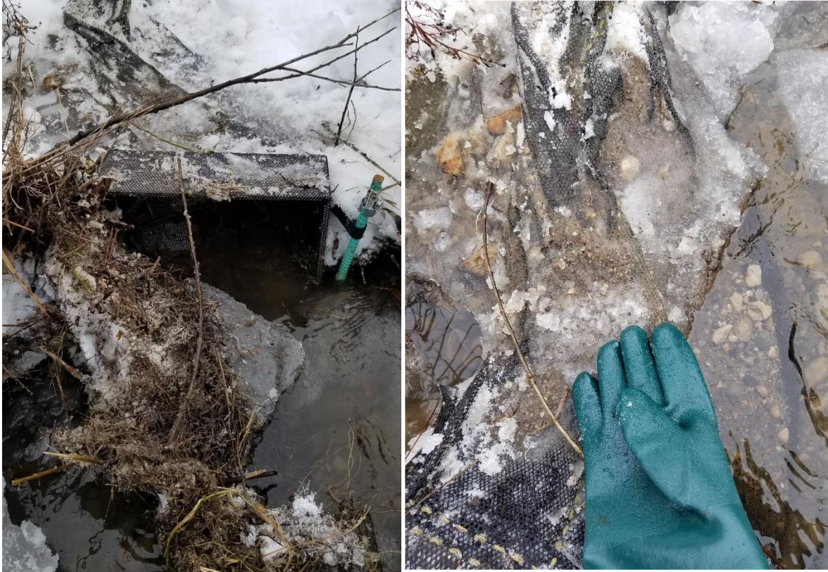
Figure 52. Bunte sediment trap sealed by ice and vegetation on January 24, 2020. (A) Ice and vegetation removed from trap opening. (B) Sand and gravel substrate found resting on top of sediment trap netting.
