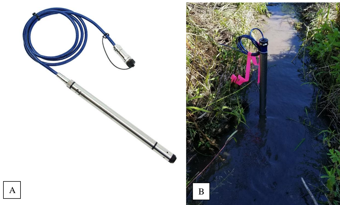
Figure 17. Seametrics PT2X pressure sensor. (A) Sensor and cable connection. Retrieved from: https://www.nexsens.com/products/sensors/water-level/seametrics-pt2x-water-level-loggers . (B) Well housing.
