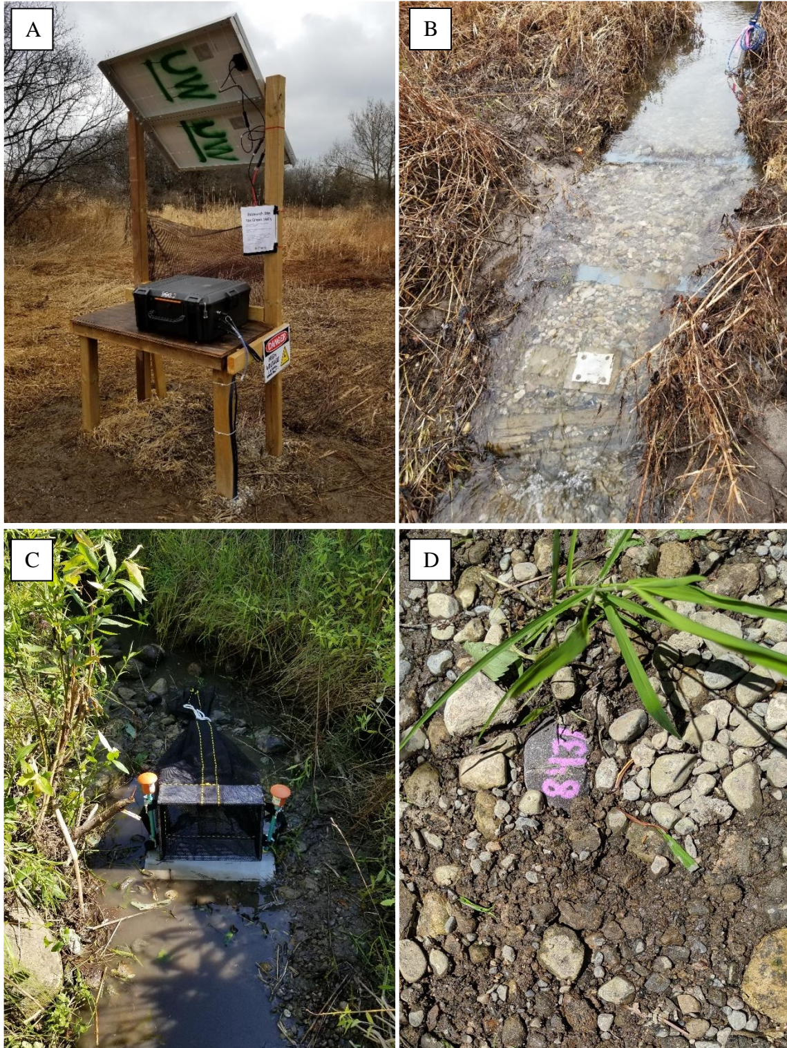
Figure 33. Carruthers Creek bedload monitoring station. (A) Tabletop frame, solar panels, and electronic equipment enclosure located within river-left overbank zone. (B) View facing upstream showing water level sensor (top-right), in-stream antenna (centre) and impact plates (bottom). (C) View facing downstream showing sediment trap. (D) Seeded tracer stone (photo credit: Bruce MacVicar).
