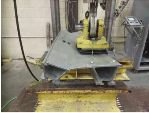
(a) Top flange ruptured.
