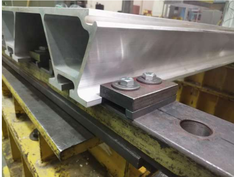
Figure 3.2: Support clamps for preventing uplift of the beam.
