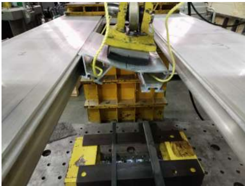
(a) Groove side connection failed.
