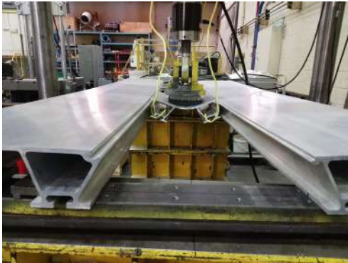
(a) Supports were bending.
