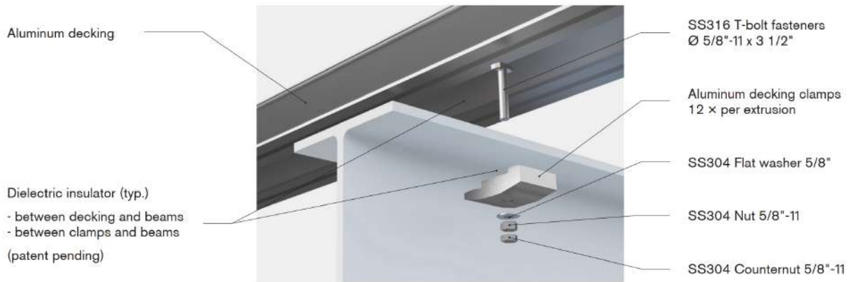
Figure 3.4: Layout of the GuarDeck® DG connection [12].
