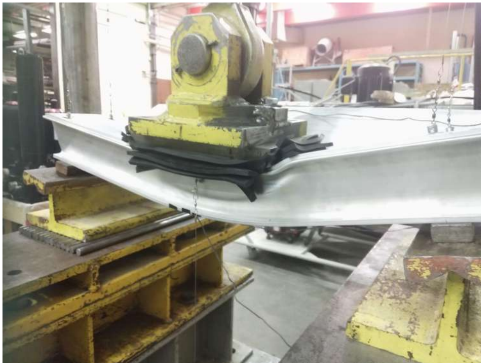
Figure 4.10: Buckled web under point load.
