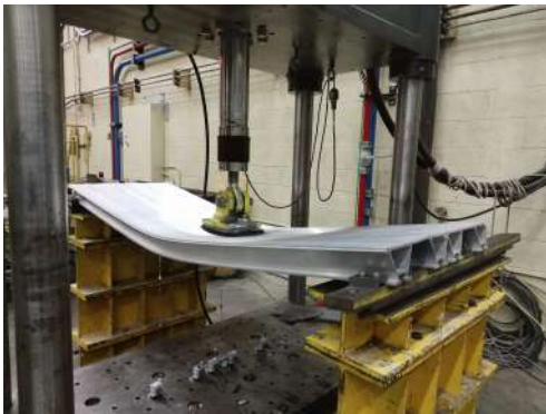
(a) Failed beams.
