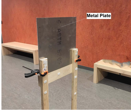
(a) Metal plate used for \Gamma_{m-short} measurement.
