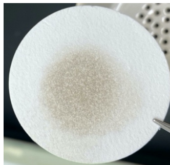
Figure 2-14: SiNWs retained on the paper filter after vacuum filtration.
