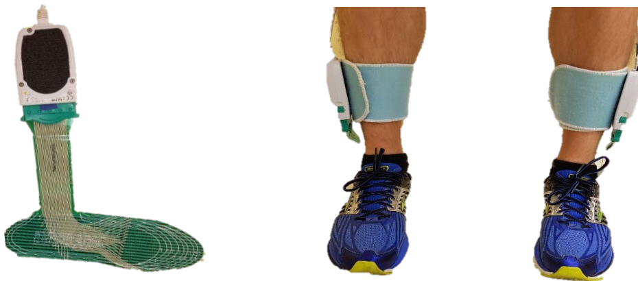
Figure 3.1: F-Scan system: A plantar pressure insole sensor (left) and sensors worn in shoes (right).
