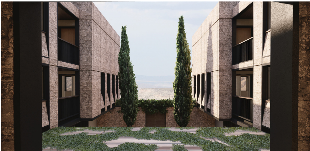
Figure 3.53 View of the konak courtyard from the central staircase. Hallways connecting the rooms are open to the outside and building envelope is established at the room level. Digital rendering.
