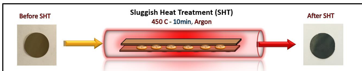
Figure (5.2) A Schematic showing optical images for the electrode surface before and after the slow heat treatment.
