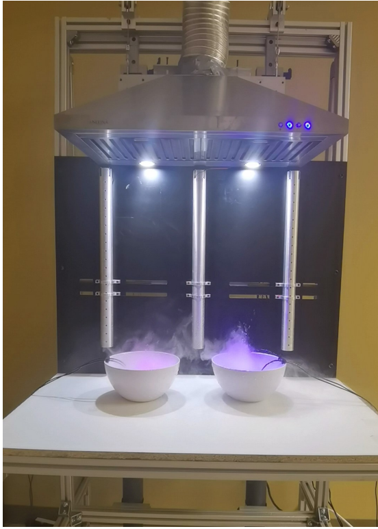
(a) Turning on the range hood while turning off the air jets generator.
