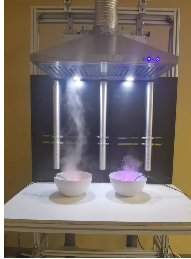
(a) Turning on middle and right jets generators. (b) Turning on middle and left jets generators.
