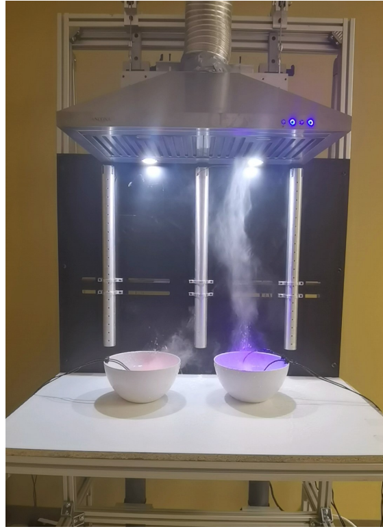
(b) Turning on both the range hood and the air jets generators (middle and right tubes).
