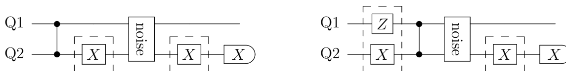
Figure 2.13: Left circuit: If it were the case that the noise existed as a separate physical process from the ideal gate, then one could target the noise directly by twirling operations (shown in dashed boxes). Right circuit: In reality the noise process is inseparable from the ideal gate, therefore we permute one of the twirling operations back through that gate to obtain the physically achievable twirling protocol.
