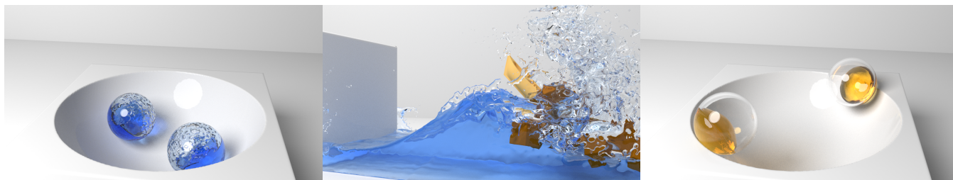
Fig. 1. Our Monolith solver enables efficient and robust two-way simultaneous rigid-rigid and rigid-fluid coupling. (Left) Two hollow glass spheres containing inviscid liquid roll around within a basin as the liquid slides and splashes. (Middle) A boat carrying multiple loads is perturbed by ocean waves. (Right) When the glass spheres instead contain viscous liquid, the no-slip boundary condition, viscosity, and friction together bring the spheres more quickly to rest.
