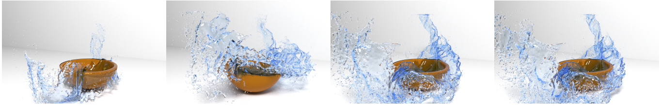
Fig. 2. Bunny-shaped inviscid liquid dropped into a bowl on the ground, with various options for pressure (P) and contact (C) coupling (see §6.1). (Left) P-C solve (decoupled). (Middle left) C-P solve (decoupled). (Middle right) PC-iterative solve (iterated weak coupling). (Right) Our proposed PC-unified solve (strong coupling). P-C solve violates fluid incompressibility, causing volume loss. C-P solve violates solid non-penetration, causing spurious oscillatory motion of the bowl. While both PC-iterative and PC-unified solves correctly preserve volume and handle bowl-ground contacts, PC-unified is approximately 10× faster.
