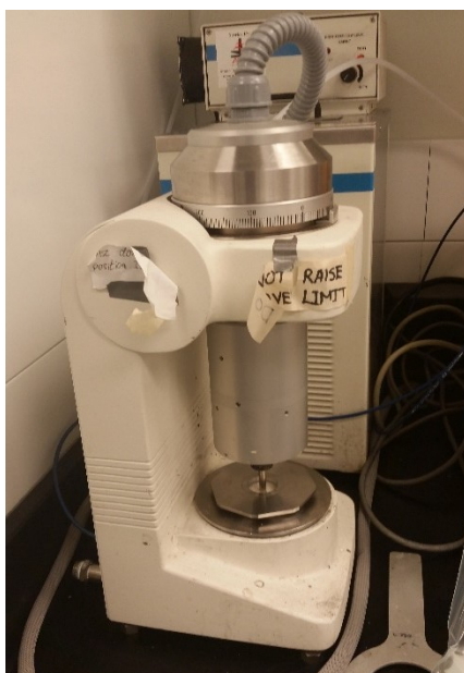
Figure 5 Bohlin CS Rheometer with C25 cup-and-bob geometry measuring the viscosity of a composite GelMA/nHA material.
