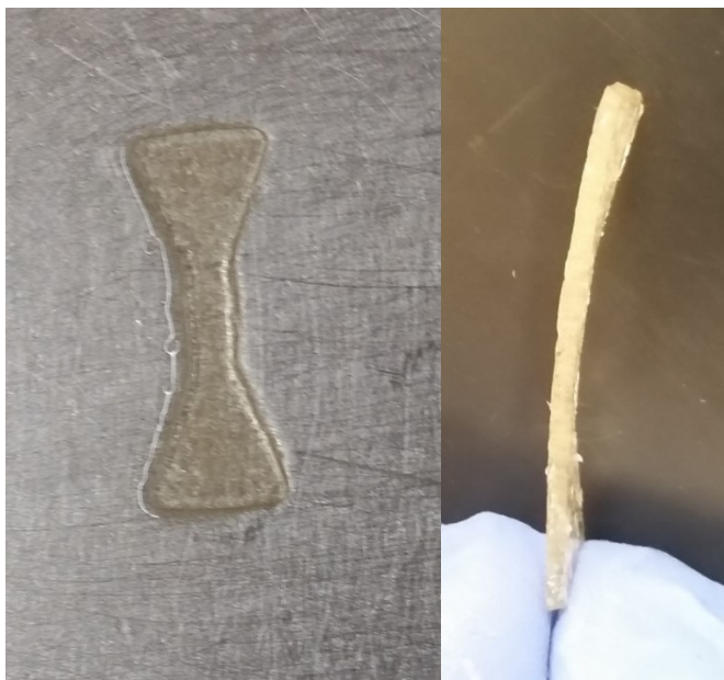
Figure 18 A dogbone of cured 1M 5X GlcN-MA/GelMA/CaCl 2 hydrogel material printed on a Phrozen mSLA printer.
