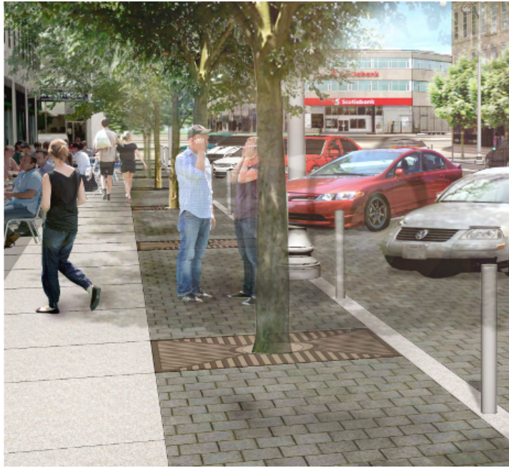
Figure 14: Design rendering of tactile paving treatments (City of Guelph, 2014)
