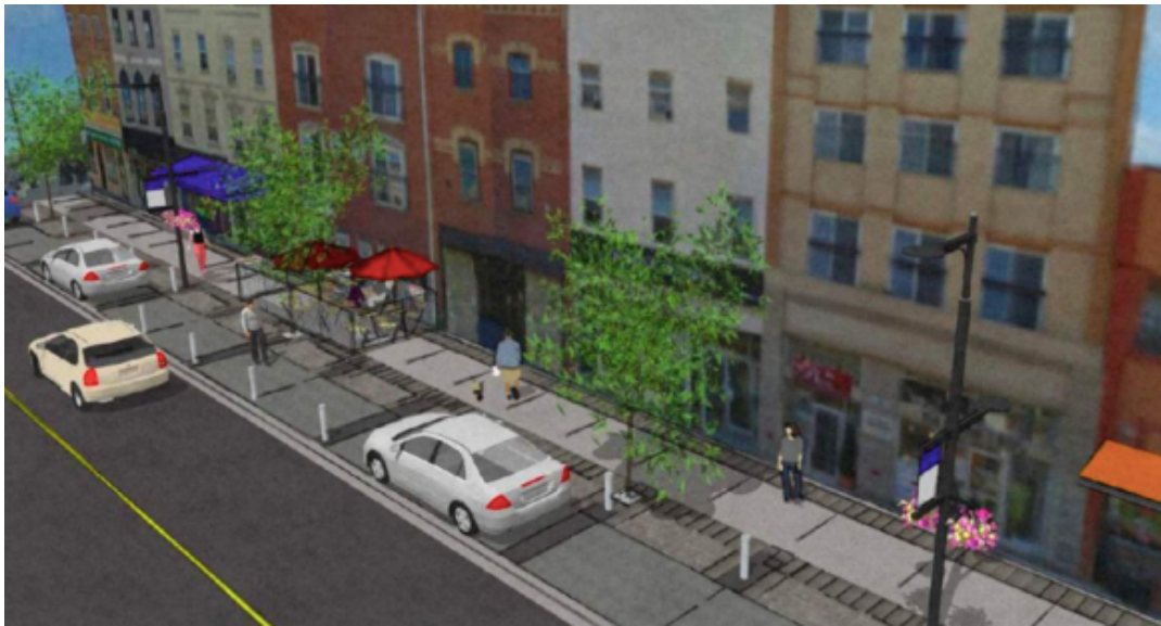
Figure 12: Design rendering of removable bollards delineating space for different uses (City of Barrie, 2019)
