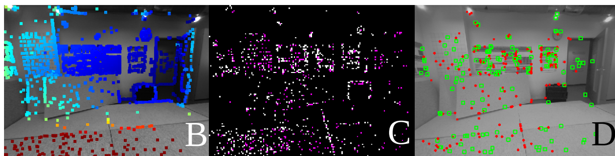
Figure 5.1: UFVO : A– shows the 3D recovered map and the different types of points used: green points contribute to both geometric and photometric residuals, red points geometric residuals only, blue points photometric residuals only and black points are marginalized (do not contribute any residuals). The blue squares are hybrid keyframes (contains both geometric and photometric information), whereas red squares are Indirect Keyframes whose photometric data was marginalized. B– shows the projected depth map of all active points. C– shows the occupancy grid which we use to ensure a homogeneously distributed map point sampling process. The white squares correspond to the projected map points while the magenta squares represent newly extracted features from the newest keyframe. Finally D– shows the inlier geometric features (active in green and marginalized in red) used during tracking (Figure better seen in color).
