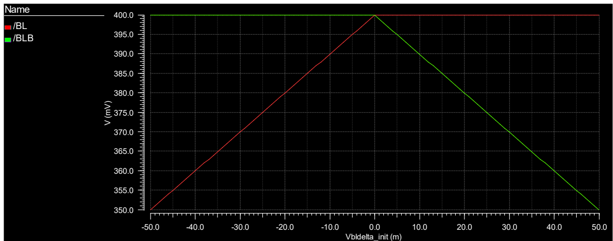
Figure 3.9 V_{BL} and V_{BLB} Setup vs \Delta V_{BL} ( V_{DD}=400\text{mV} )
