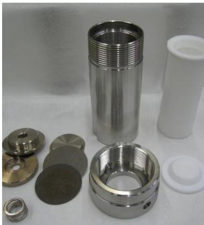
Figure 2.1 Pressure Vessel for solvothermal NCs synthesis, including stainless-steel shells and lids, teflon cups, and bursting discs.
