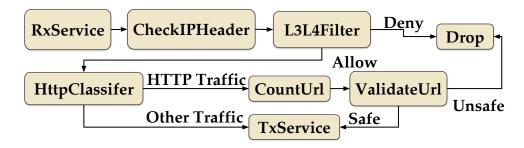
Figure 2.17:  $\mu$ NF realization of the SFC from Figure 2.3(a)
