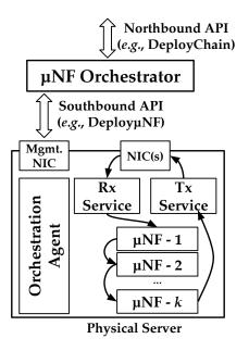
Figure 2.5: System components
