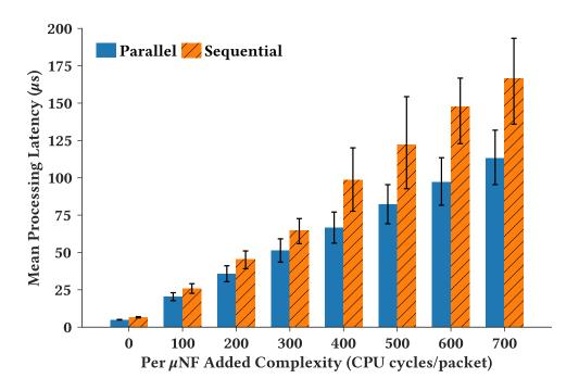
Figure 2.13: Impact of parallelism in  $\mu$ NF processing graph
