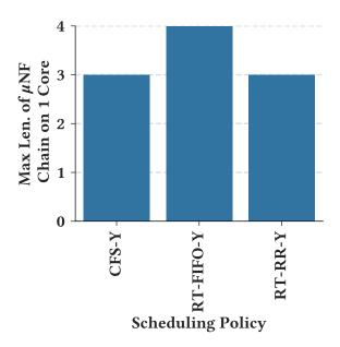
Figure 2.9: Maximum length of a  $\mu$ NF chain able to sustain line rate (64B) while sharing a core
