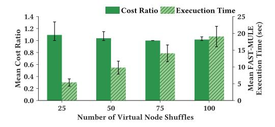
Figure 3.8: Impact of virtual node shuffle on FAST-MULE's performance
