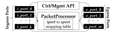
Figure 2.6:  $\mu$ NF architecture
