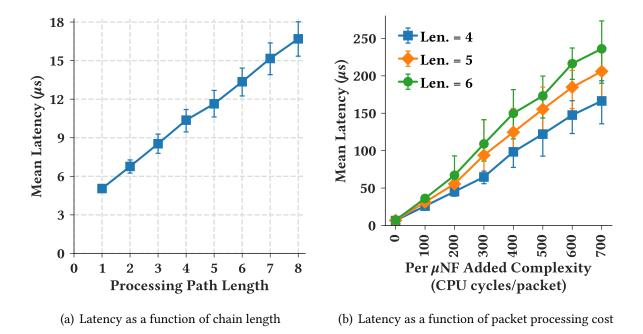
Figure 2.14: Impact of  $\mu$ NF processing path length
