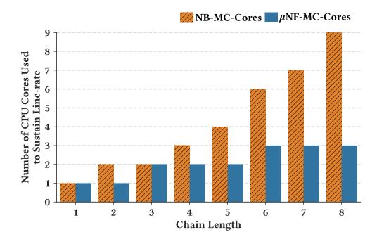
Figure 2.16:  $\mu$ NF vs. NetBricks [1]: number of CPU cores used
