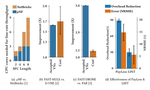
Figure 1.3: Highlights of thesis contributions: (a) effectiveness of  $\mu$ NF in enabling finer-grained resource allocation compared to NetBricks [1]; (b) VN acceptance and embedding cost comparison between FAST-MULE and D-VNE [2]; (c) VN acceptance and embedding cost comparison between FAST-DRONE and PAR [3]; and (d) effectiveness of PayLess and LINT in reducing control and data plane overhead, respectively.
