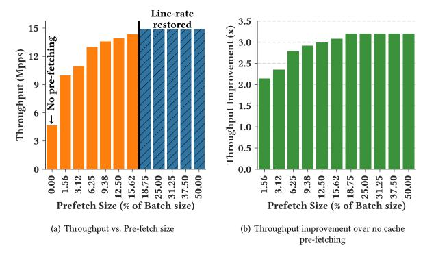
Figure 2.12: Impact of pipelined cache pre-fetching
