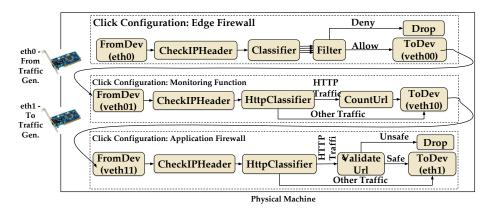
(a) Monolithic VNFs chained with veth pairs (configuration-(i))
