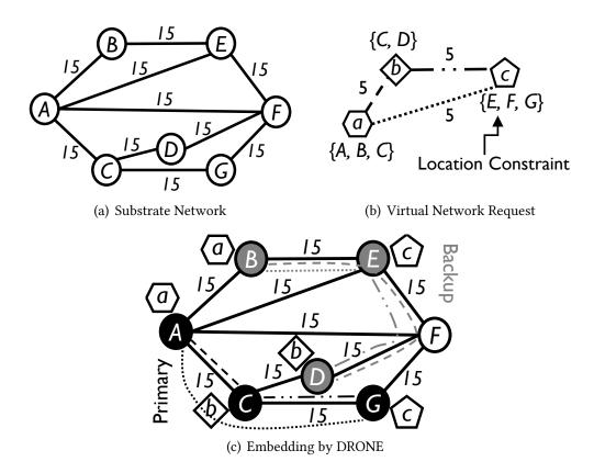
Figure 4.1: Example VN embedding with DRONE
