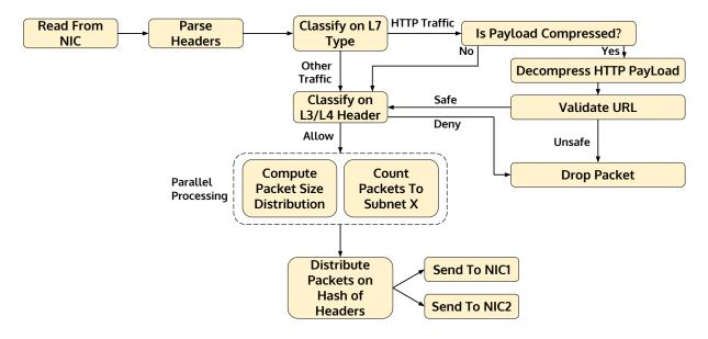
Figure 2.4: Microservice-based realization of the SFC from Figure 2.2(a)
