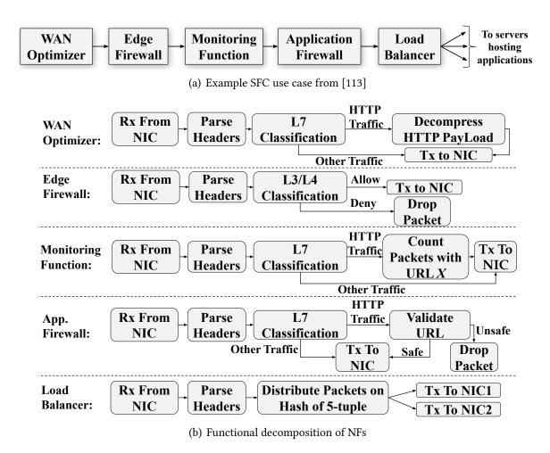
Figure 2.2: Common packet processing tasks across NFs
