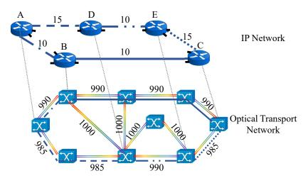
Figure 3.1: Multi-layer IP-over-OTN substrate network
