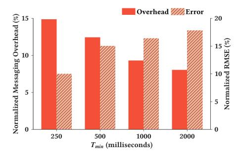
Figure 5.7: Overhead and measurement error
