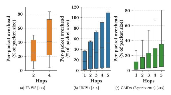
Figure 5.8: Packet size increase due to INT
