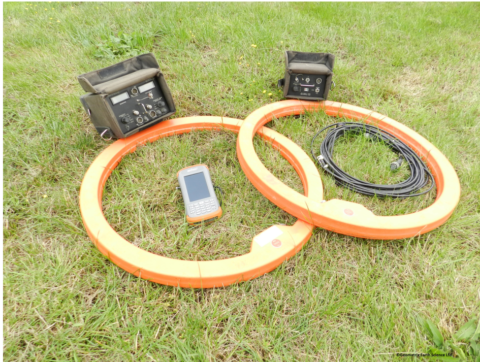
Figure 4.3: Geonics EM-34 Ground Conductivity Meter system. (Geomatrix LTD Undated
