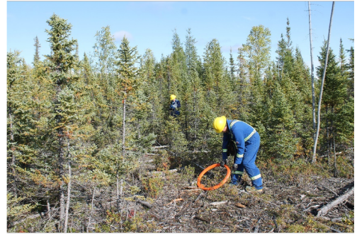
(b) Setting up the EMI (Geonics EM-34) system at the MW04T site.
