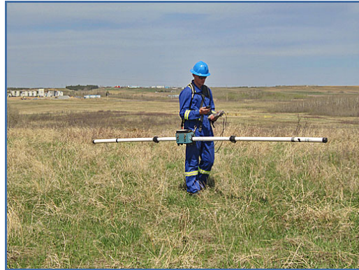
Figure 4.2: Geonics EM-31 Ground Conductivity Meter system. (Magna Enterprises Undated)
