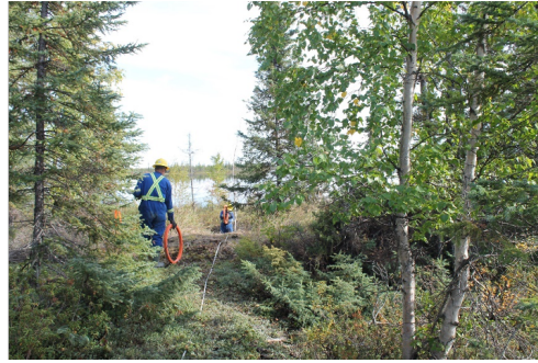
(c) Setting up the EMI (Geonics EM-34) system at the Marg Lake site.
