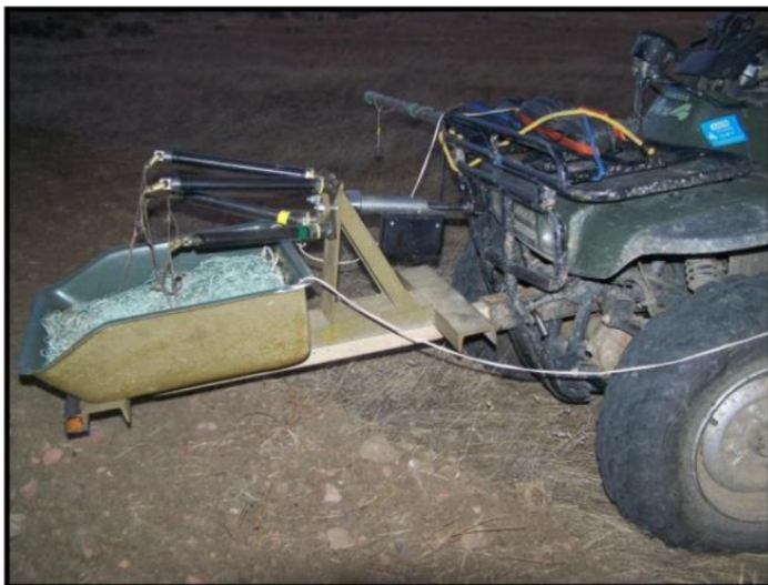
Figure 2.3: Bumper-mounted CODA (CODA Enterprises, Mesa, AZ, USA) net launcher on ATV. We developed this method to capture greater sage-grouse in Wyoming, USA, during spring and autumn 2008–2011.
