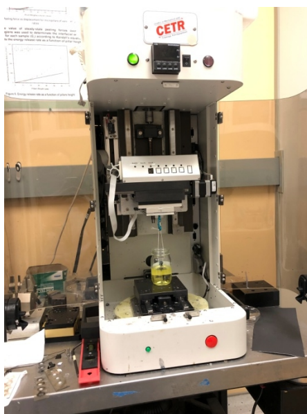
Figure 21 Dip coating setup (A tensile tester with z-axis motorized stage)
