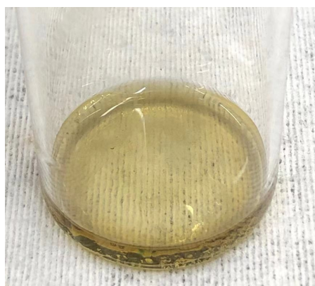
Figure 39 Picture of tin oxide ink made from tin oxide sol
