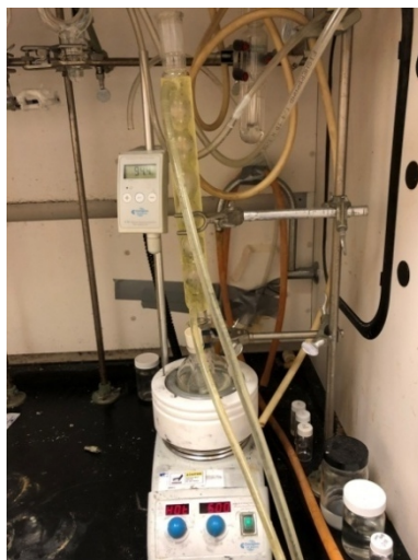
Figure 19 Experimental setup for synthesizing tin oxide sol
