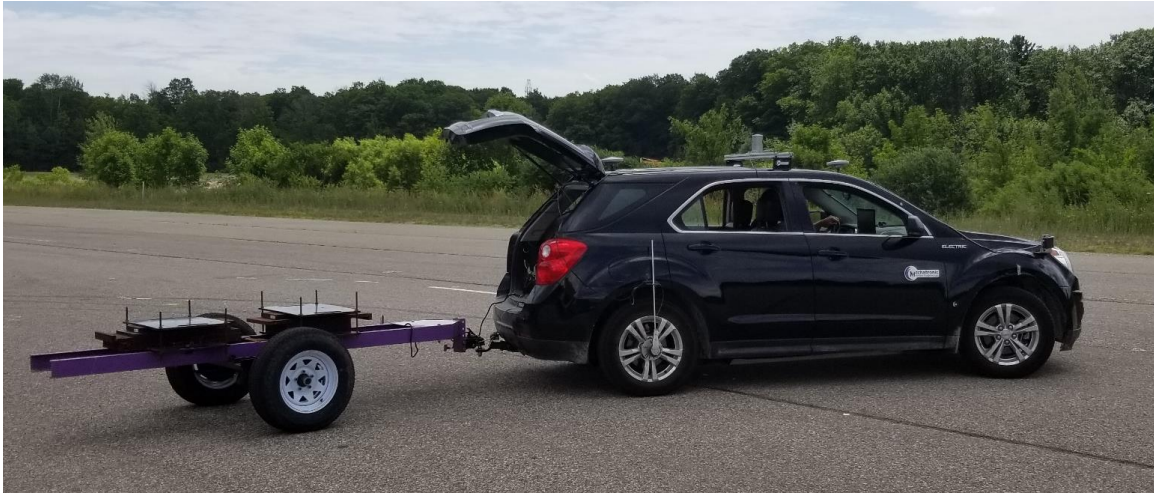
Figure 4.16: The electric all-wheel-drive Chevrolet Equinox vehicle and the trailer attached
