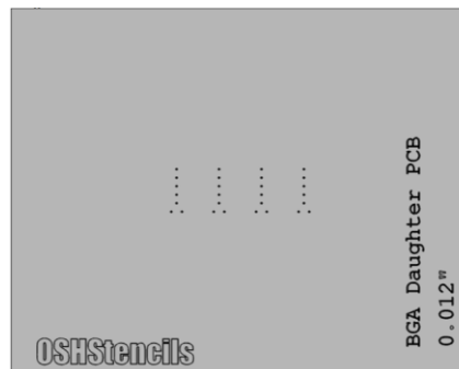
Figure 2.12: Illustration of daughterboard stencil. Stencil was manufactured using stainless steel. Dimensions are 2.162 inches by 1.712 inches, with a thickness of 4 mils. Stencil holes have a diameter of 12 mils.
