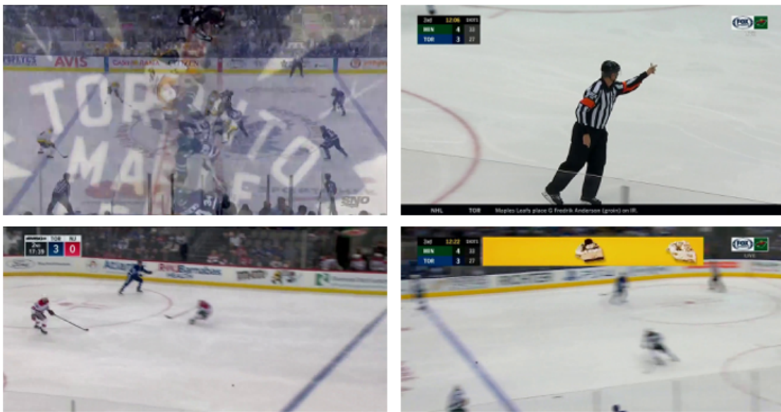
Figure 3.7: Failure modes for the hockey homography annotation tool. Clockwise from top left: ice blocked by broadcast graphic; too zoomed in, not enough high fidelity keypoints; motion blur; area around blue line, too few high fidelity keypoints.
