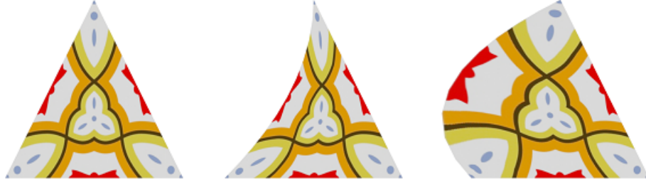
Figure 4.5: A triangle mapped harmonically to fill a patch of fabric that includes a boundary segment.
