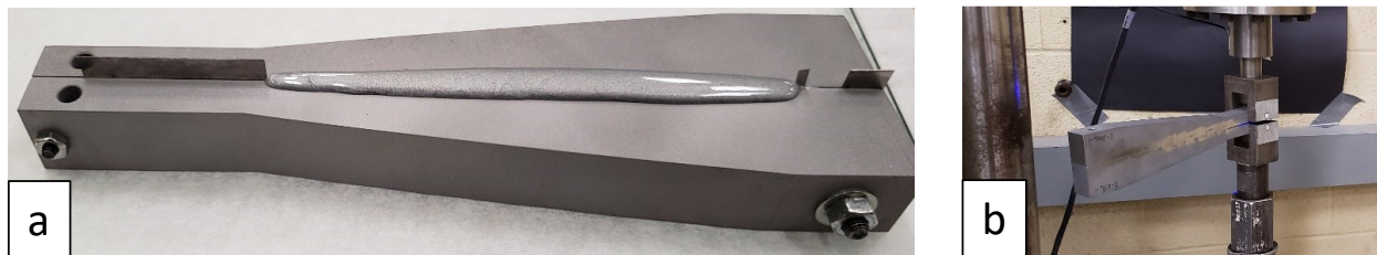
Figure 36: Assembly of TDCB specimen (a), and TDCB test (b)
