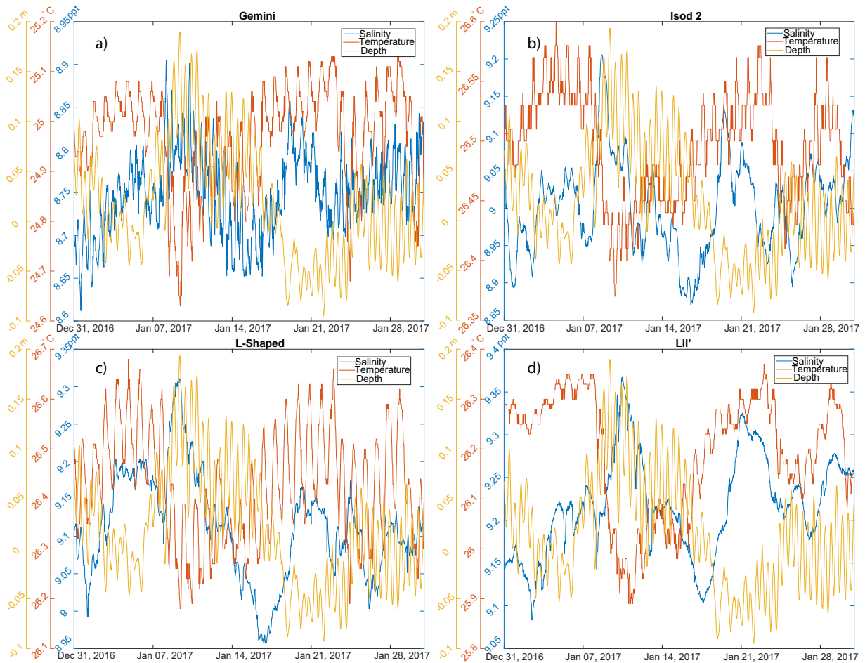
Figure 2.9: The salinity, temperature and water depth measurements at the sensor locations during a rainfall event in January 2017. (a) Gemini, (b) Isod 2, (c) L-Shaped, and (d) Lil'.
