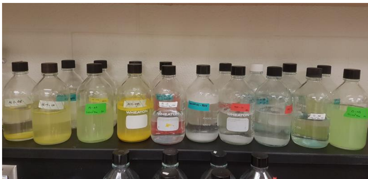
Figure 4.19: Stock suspensions of PE, PEEK, PS and ACR microplastics in MilliQ™ water, electrolyte solution, Grand River water, and Lake Ontario water.
