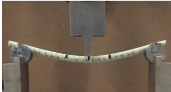
Figure 3.21: M20 Bar in 3-Point Bending Test Before Failure
