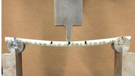
Figure 3.19: Deflected M20 Bar Shortly After Start of 3-Point Bending Test
