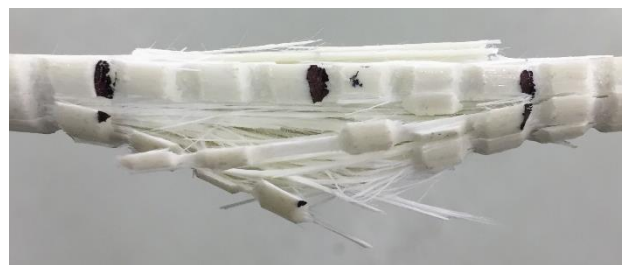
Figure 3.40: Close-up View of Side Face of M15 Specimen Subjected to 4-Point Bending
