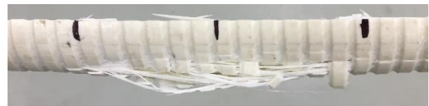
Figure 3.44: Close-up View of Side Face of M32 Specimen Subjected to 4-Point Bending
