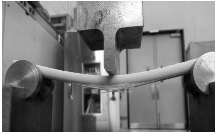
Figure 2.7: 3-Point Bending Test of GFRP Specimen (Arczewska, 2017)
