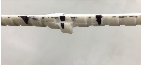
Figure 3.37: Close-up View of Side Face of M13 Specimen Subjected to 3-Point Bending
