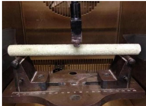
Figure 2.4: FRP Specimen with Full Cross-section Tested in 3-Point Bending Test (Maranan et al., 2014)
