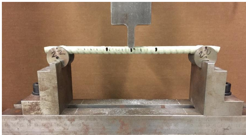
Figure 2.6: Front View 3-Point Bending Test Specimen with Longitudinal Cut
