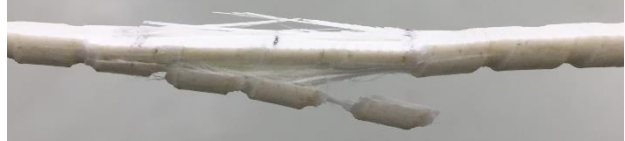
Figure 3.36: Close-up View of Side Face of M8 Specimen Subjected to 4-Point Bending
