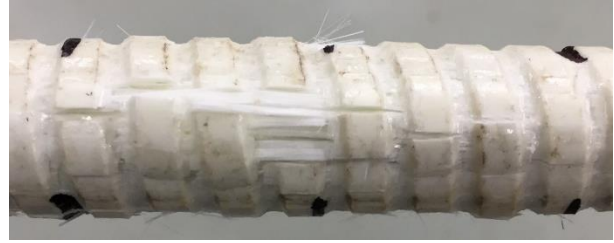
Figure 3.30: Close-up View of Bottom (Tensile-Stressed) Face of M20 Specimen in 4-Point Bending
