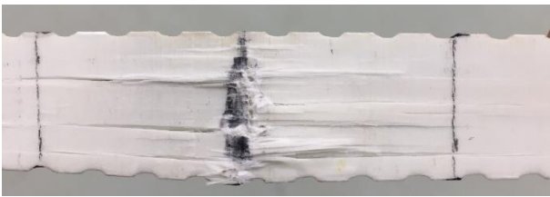
Figure 3.33: Close-up View of Top (Compressive-Stressed) Face of M20 Specimen Subjected to 3-Point Bending
