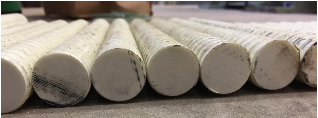
Figure 3.11: Close-up View of GFRP Bars Prior to Longitudinal Cut
