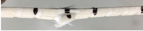
Figure 3.35: Close-up View of Side Face of M8 Specimen Subjected to 3-Point Bending
