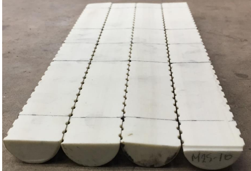
Figure 3.13: Close-up View of GFRP Bars Post-Longitudinal Cut
