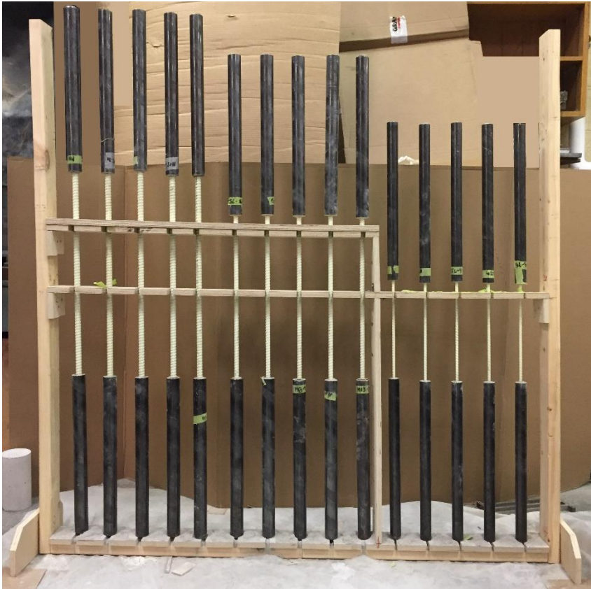
Figure 3.16: Tensile GFRP Specimens in Casting Stand
