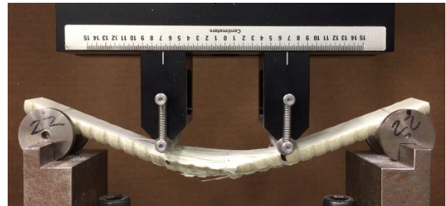
Figure 3.24: M20 Bar in 4-Point Bending Test After Failure
