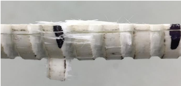
Figure 3.31: Close-up View of Side Face of M20 Specimen Subjected to 3-Point Bending
