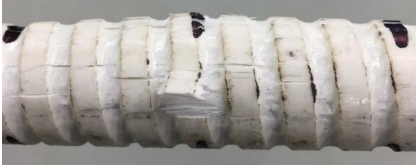
Figure 3.29: Close-up View of Bottom (Tensile-Stressed) Side of M20 Specimen Subjected to 3-Point Bending
