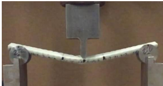
Figure 3.23: M20 Bar in 3-Point Bending Test After Failure
