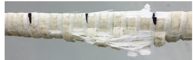
Figure 3.42: Close-up View of Side Face of M25 Specimen Subjected to 4-Point Bending
