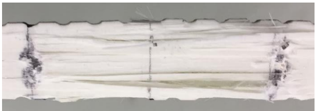
Figure 3.34: Close-up View of Top (Compressive-Stressed) Face of M20 Specimen Subjected to 4-Point Bending
