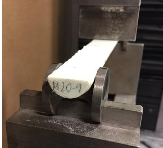
Figure 2.5: Side View 3-Point Bending Test Specimen Cut Longitudinally
