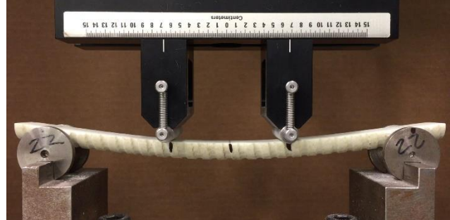
Figure 3.20: Deflected M20 Bar Shortly After Start of 4-Point Bending Test
