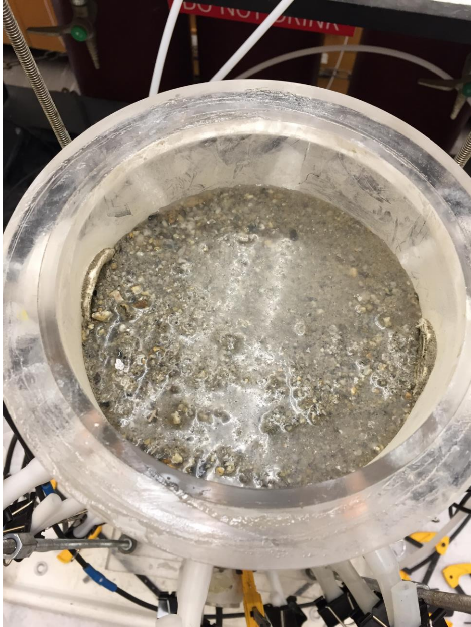
Fig. B.4 Standing water at the top of Diavik matrix material in the column during the end of the initial wetting process.
