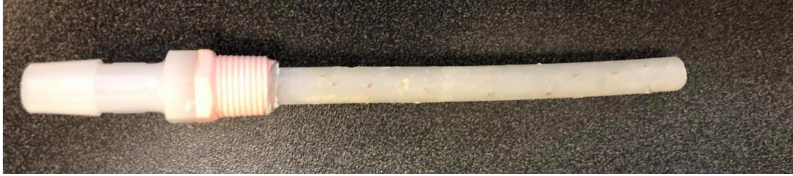
Fig. B.2 Single diffusion port (10 cm length) to allow for gaseous diffusion into the column. Polyethylene tubing perforated radially along the length (6 cm) of the tube with a thumb tac.
