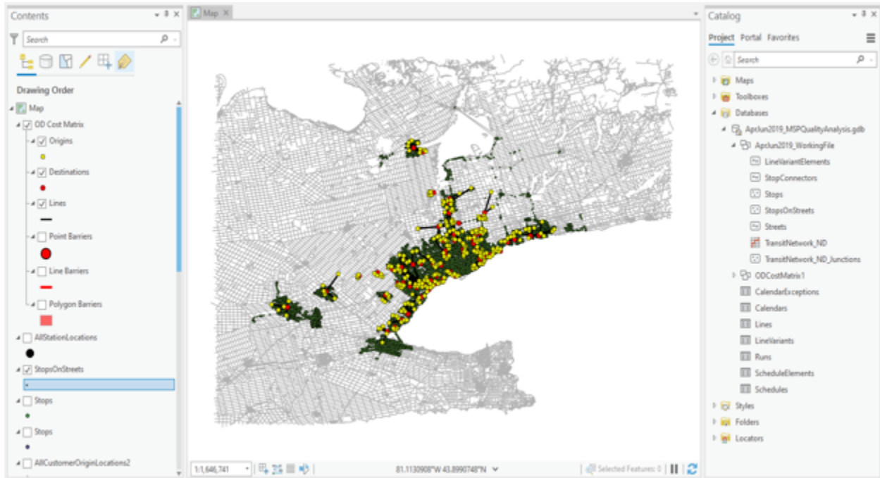
Figure 11 - Virtual Transit Network of All Municipal Service Providers in the Greater Golden Horseshoe, Used to Obtain Feeder Bus Connection Quality (ex. Travel Time) Estimates
