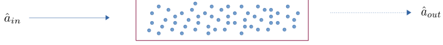
Figure 4.6: 1D propagation through a medium can be expressed via input and output field operators.[226, 233]
