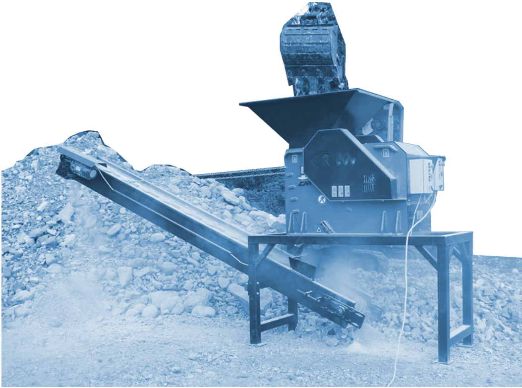
Figure 39 Mini electric jaw crusher CR series is ideal for the recycling of aggregates from small demolitions. (CM Crusher Machines, 2020)
