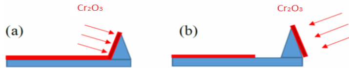
Fig 3.6 Tip after 60° angle deposition from both (a) front, and (b) opposite side of the tip
