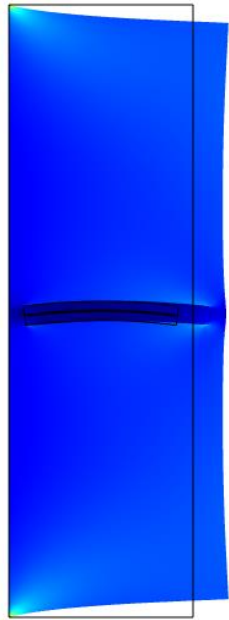
Figure 4.31 Overexaggerated Stress Deformation from Tensile Stress
