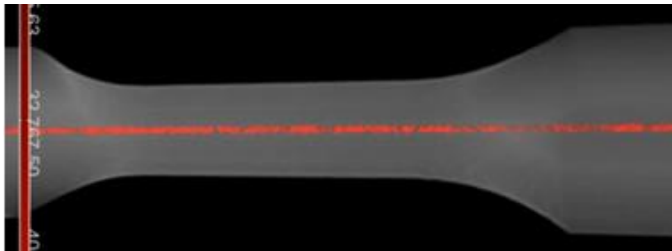
Figure 4.1 CT Scan of 400 Micron Channel in Tensile Coupons
