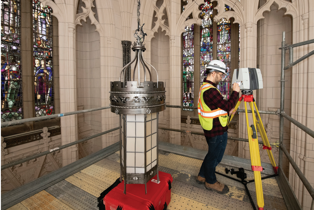
Figure 30 A worker scans the Memorial Chamber with a laser scanner in January 2020
