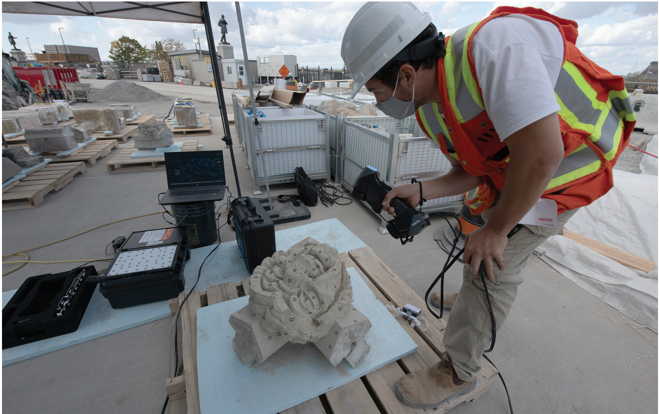
Figure 34 A digital imaging specialist does a 3D scan of a stone carving removed from the Senate porch entrance
