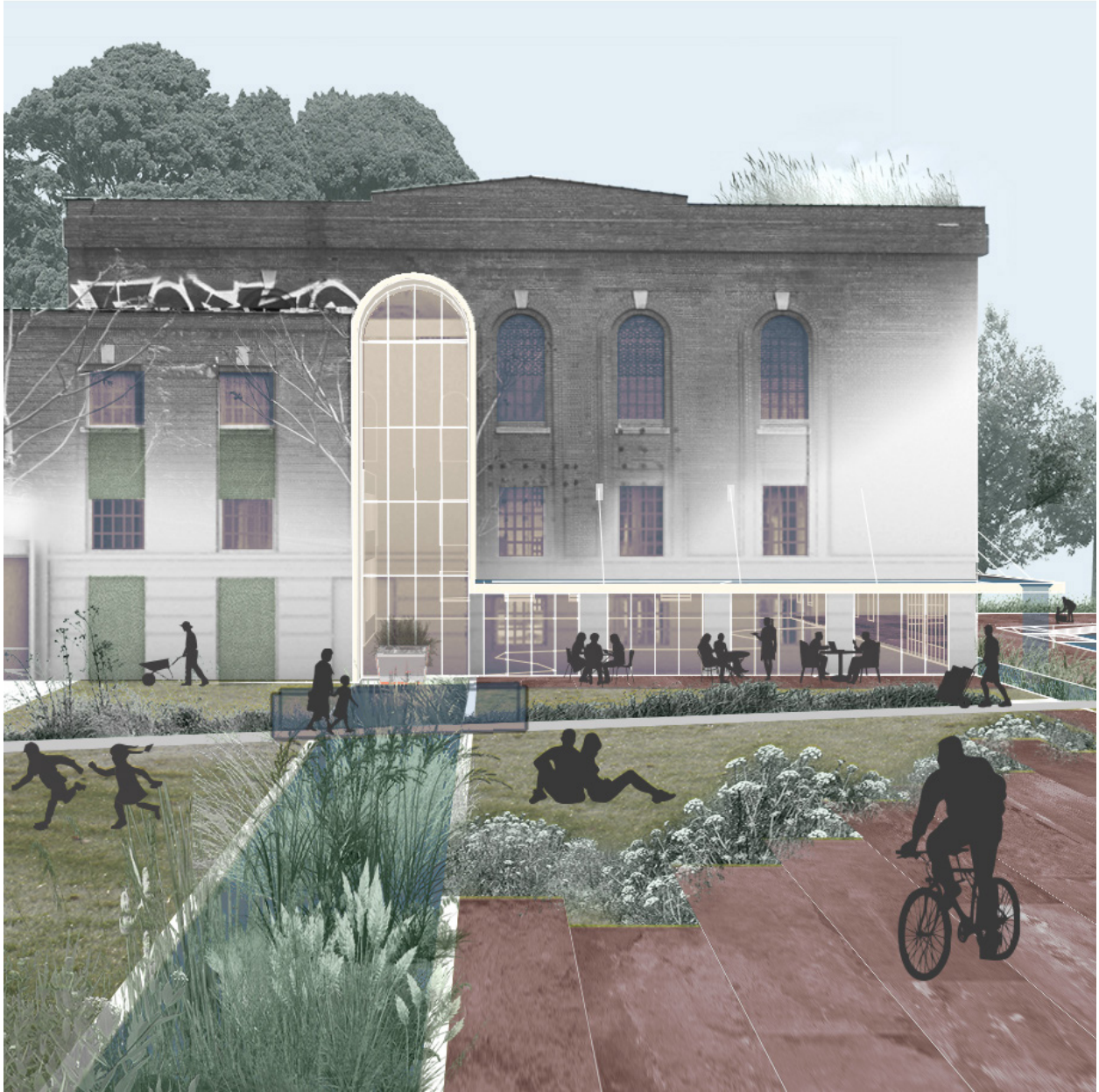
5.45 _ West Elevation Showing Bio filtration Swale, Permeable Paving and Cafe Overhang Stormwater Roof Addition
