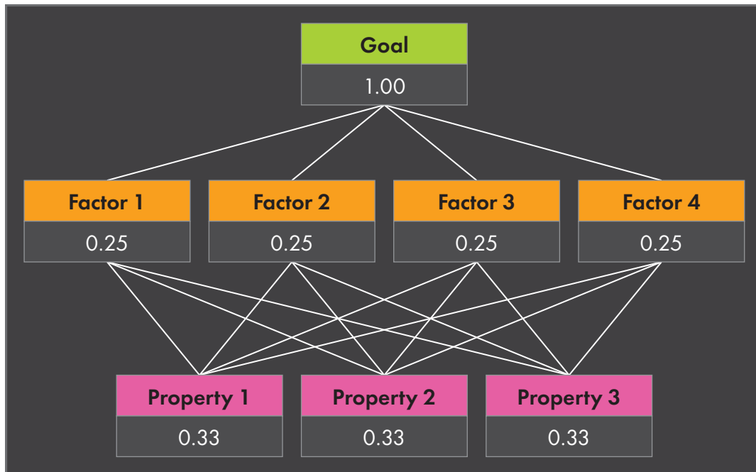
Figure 2.3.c: Simple analytic hierarchy process structure, based on diagram by Sander (2009), redrawn by author.
