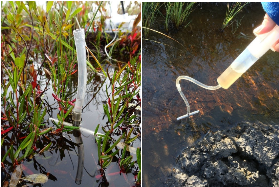
Figure 7: Photos of the PushPoint sampler unit showing positive hydraulic head at a discharge location (left) and using a syringe to obtain samples below surface water (right). Photo on the left was taken by Brewster Conant Jr.
