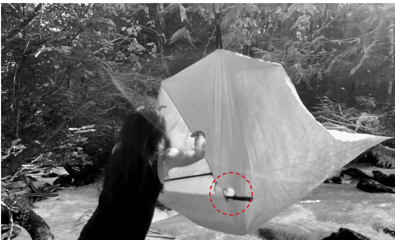
FIG 4.28 Failure of the membrane at right corner where pole handle applies pressure to the membrane (centre).
