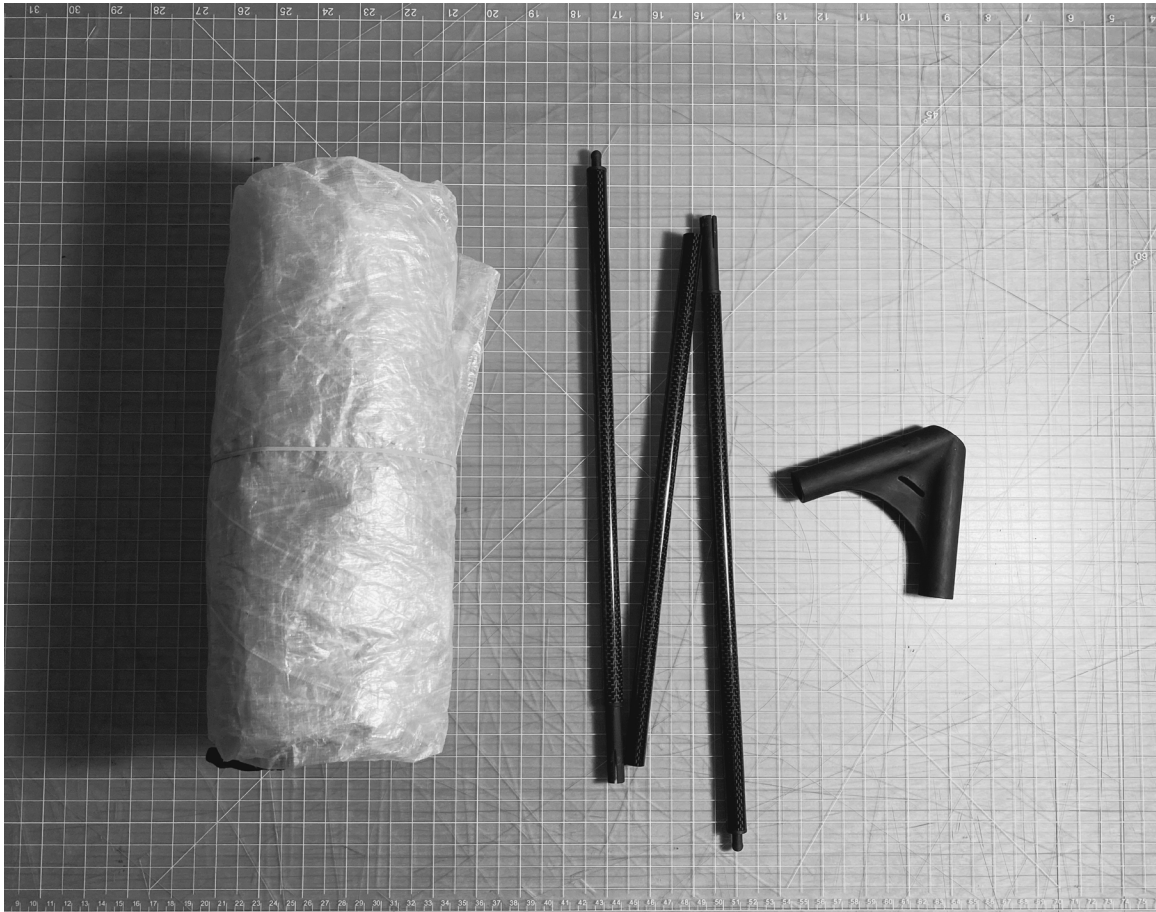
FIG 4.43 The completed components of the shelter system: enclosure, ridge pole, and pole connector.
