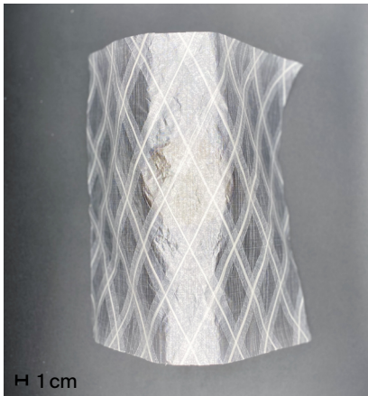
FIG 4.09 Comparison of buckling resistance in parallel tape reinforcing and intersecting tape reinforcing.
