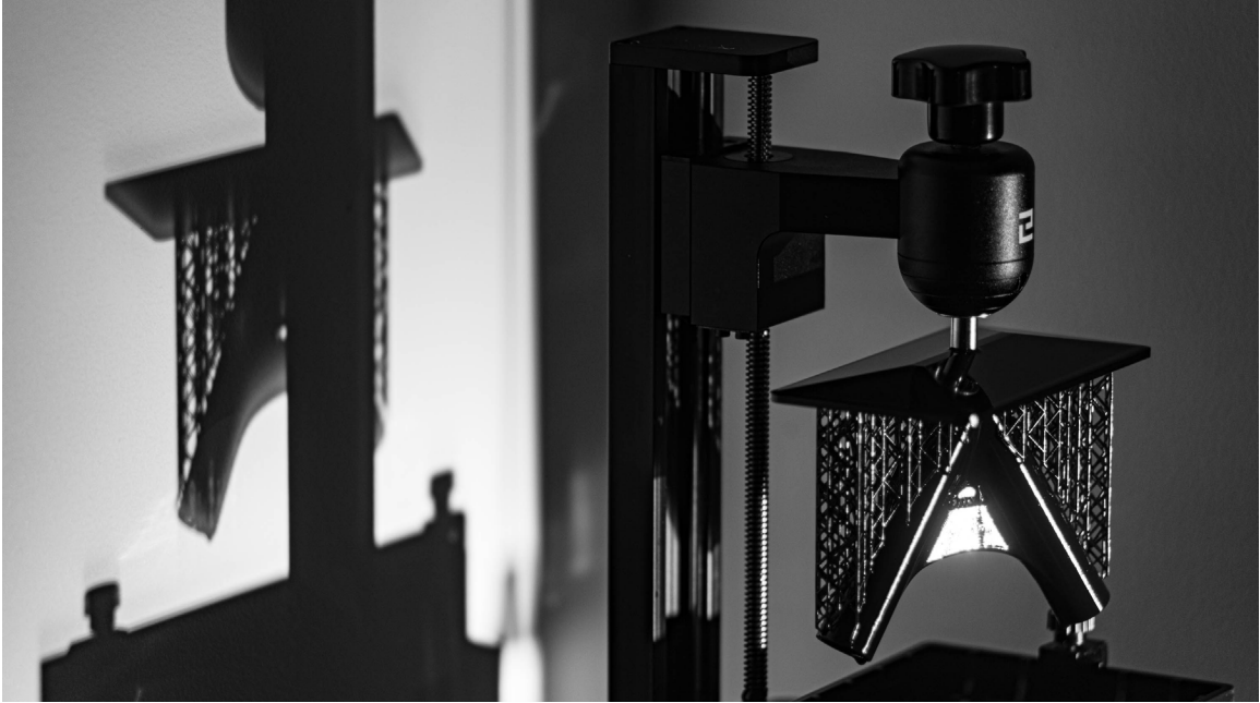
FIG 4.42 3D Printing the final 'V' joint connector.
