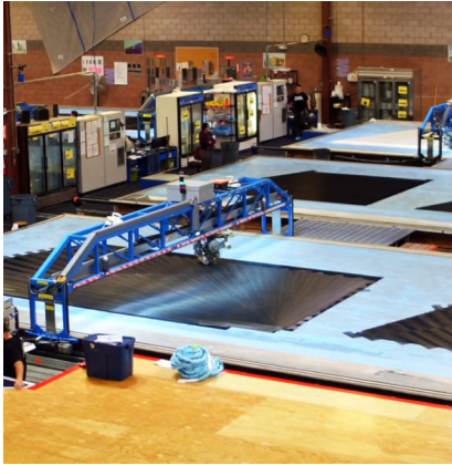
FIG 5.14 Large CNC beds of the North Sails Automated Taping System (ATS).
