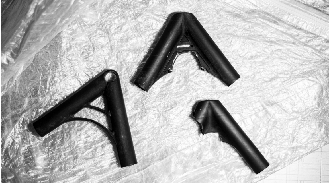
FIG 4.41 Previous iterations of the 'V' joint connector.
