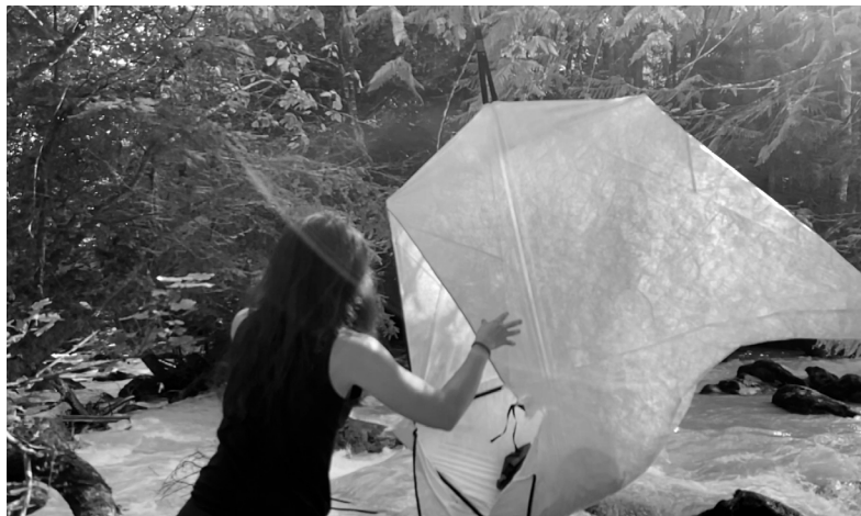
FIG 4.31 Despite regional failures in the membrane, the top anchor remained intact.
