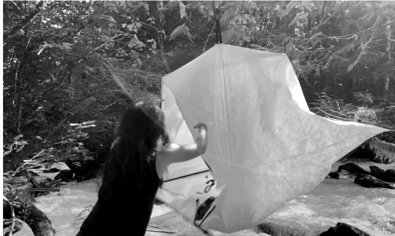
FIG 4.29 Failure of membrane at right corner created substantial springback in pole 'V' connector.
