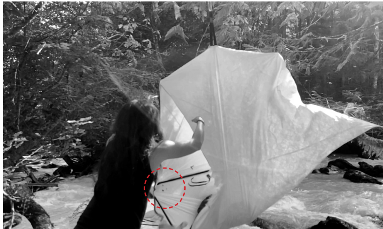
FIG 4.30 Springback causes 'V' connector to fracture and break apart.
