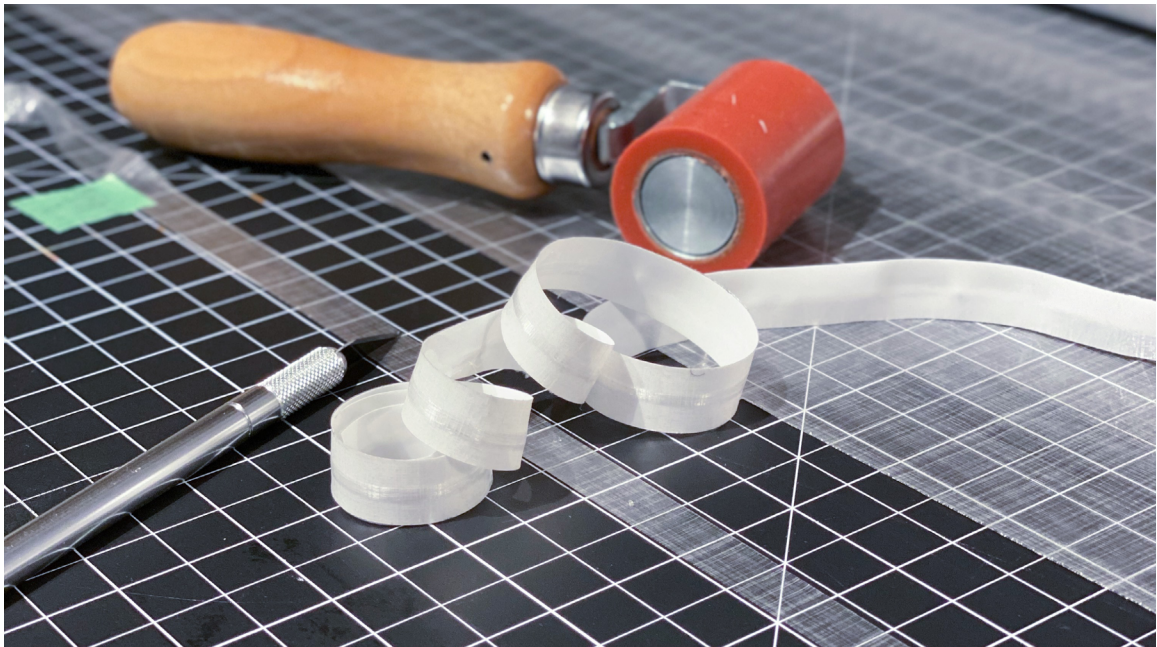
FIG 4.05 Filament tape made with double-sided PSA and DCF backing.
