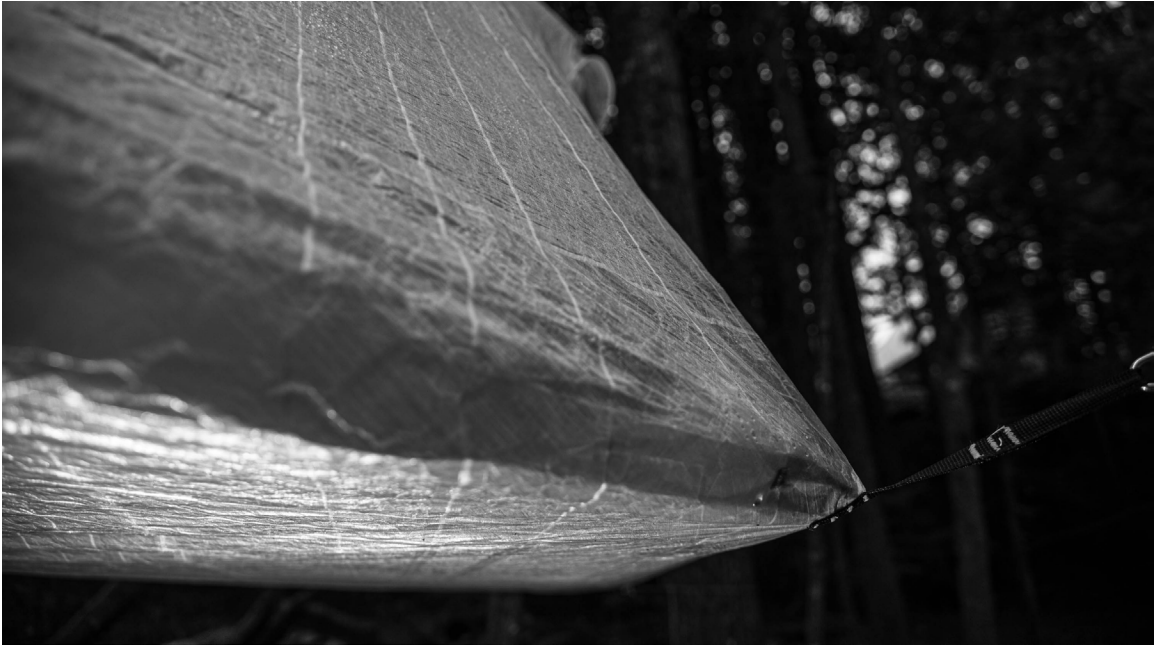
FIG 5.09 Filaments wrapping up from bottom of shelter.
