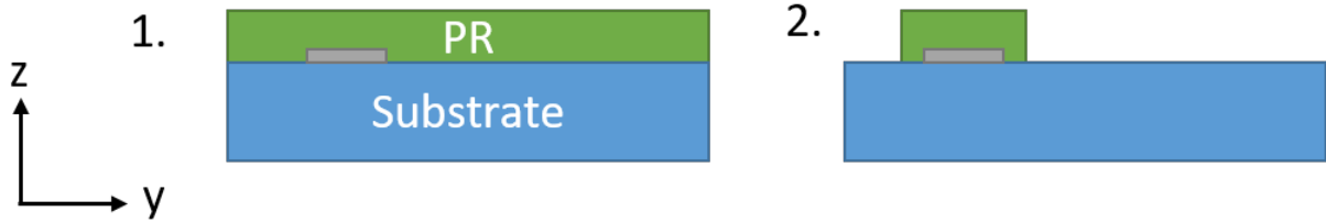
Figure 6.5: Photoresist (PR) sacrificial layer (green) patterned by UV lithography with mask 2.
