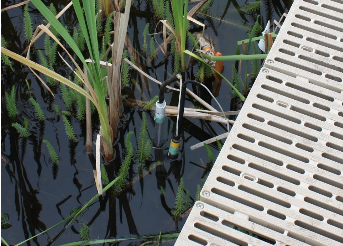
Figure 2-2 Photo of two suction lysimeters installed at 30 cm bgs (left, with white tape) and 10 cm bgs (right, with yellow tape) in a ponded area.
