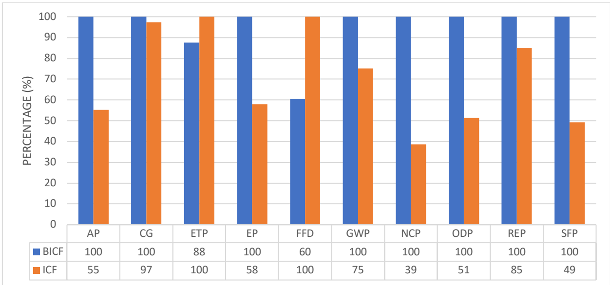
Figure 4-1 Comparison of ICF and BICF systems. The results are relative to the product with the highest impact for each indicator and impact for 1 m 2 of the ICF and the BICF
