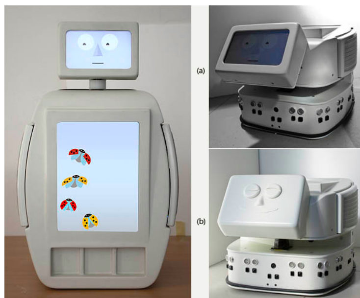
Figure 2.2: Different configurations of the IROMECC robot. (a) shows the digital face configuration, and (b) shows a static, pre-designed face. Obtained with permission (courtesy of Prof. Patrizia Marti, University of Siena).
