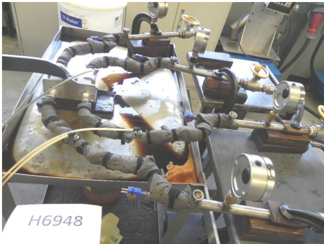
Figure 5.1: Experimental transmission oil cooler testing
