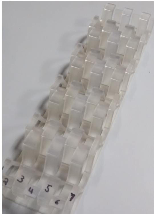
Figure 3.45: 3D printed 10:1 scale model of turbulizer
