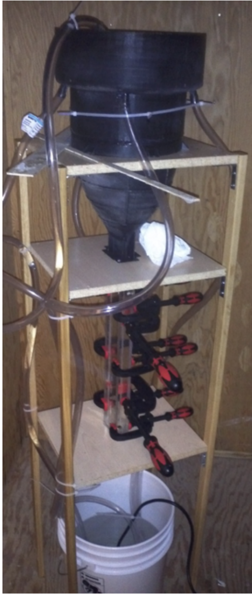
Figure 3.48: Completed water tunnel test section
