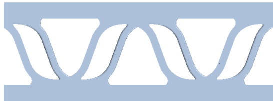
Figure 3.5: profile of 50% offset turbulizer, turbulizer blades evenly spaced along centreline
