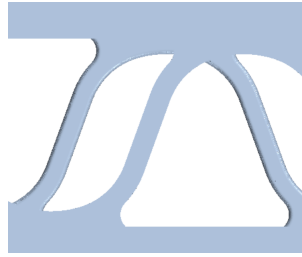
Figure 3.33: 0.1 mm channel height reduction in conjunction with 0.5 mm braze radius. The truncated radius due to coreplate extrusion can be seen in comparison to the previous figure
