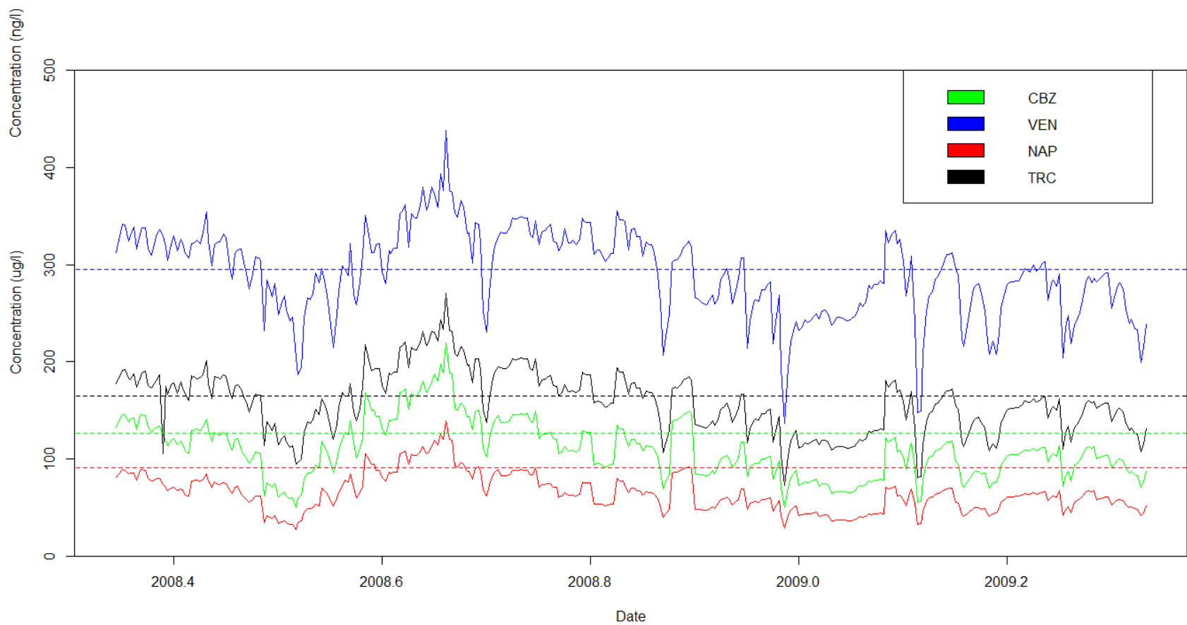
Figure 10: Kitchener WWTP train A modeled effluent TOxC concentration, pre-upgrade. Dashed lines represent observed average Kitchener WWTP effluent concentrations from 18 Nov, 2010.
