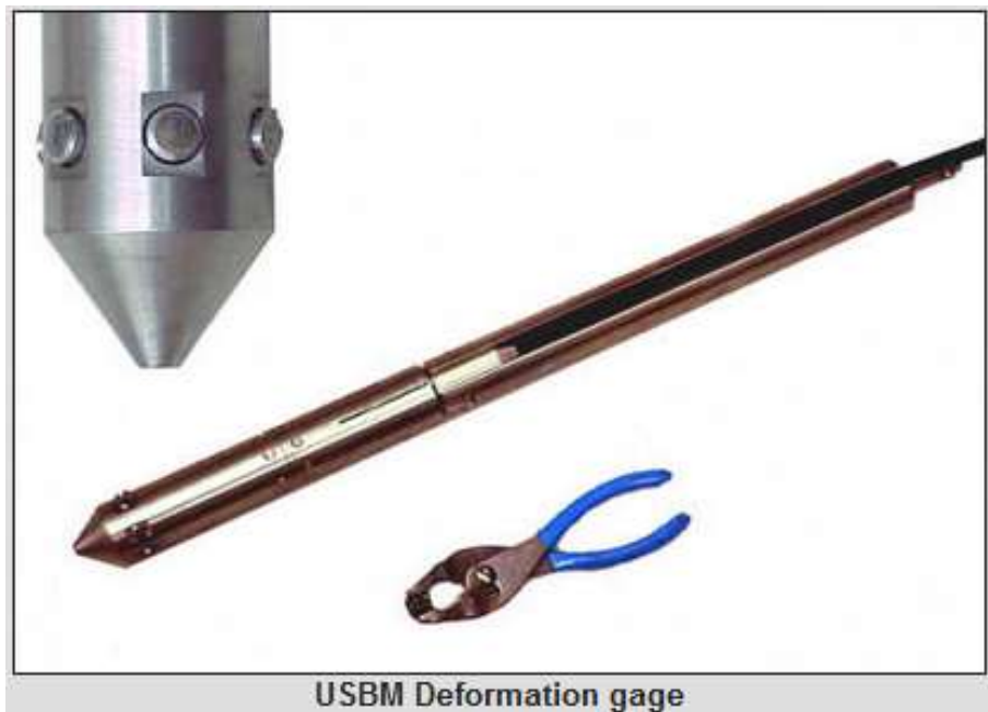
Figure 2-7: Example of deformation gage
