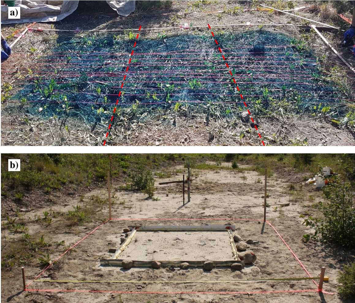
Figure 2.2: Photographs taken of the dye test setup for: a) Test 1, after dye application, facing east, with red dashed lines showing the approximate locations of furrow centerlines; and b) Test 2, prior to application, facing east. The pink strings shown in a) were used as guides for incrementally excavating the plot area.
