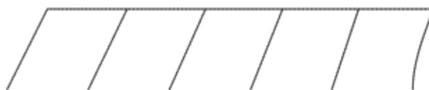
637 Figure 16 – Buckled shape of the lean-on frame in Example 2 with n = 5 bays
