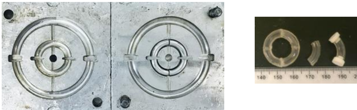
Figure 3.1: Aluminum mold for the fabrication of reservoir-type IVR segments. The mold can produce segments for a large human size IVR (55 mm outer diameter and 5.5 mm cross-sectional diameter) and a small macaque size IVR (25 mm the outer diameter and 5 mm the cross-sectional diameter). The wall thickness for both IVRs is 0.75 mm. IVR segments were fabricated using hot-melt injection molding of HP-60D-35 PU and HP-93A-100.
