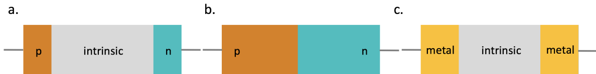
Figure 3.1: (a) Schematic of a p-i-n junction with two p-type and n-type contacts separated by an intrinsic, un-doped layer. Carriers which are generated within the intrinsic layer are separated by a field across the terminals, and drift to the contacts. (b) Schematic of a p-n junction, consisting of a p-type and n-type region. Photogenerated carriers at the junction are separated by the staggered band alignment. (c) A schematic of a Schottky-barrier diode, which is made with an intrinsic material contacted with two metals. Carriers are generated in the intrinsic region and collected by the metal contacts.
