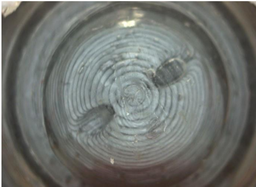
Figure 4.9. Scratched contact lens on OcuBlink 2.0. A contact lens with a scratched front surface due to dehydration of lens and eyelid during blinking at 34°C for 16 hours.
