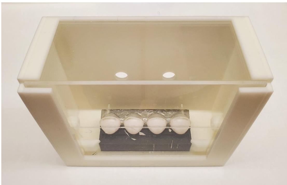
Figure 4.15. OcuBlink 3.0 XL enclosed. Acrylic sheets used to enclose the OcuBlink chamber to maintain humidity and temperature.
