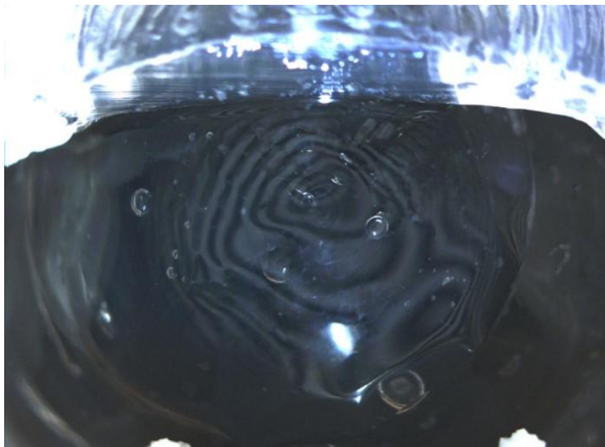
Figure 4.10. Distorted contact lens on OcuBlink 2.0. A contact lens distorted after 8 hours of blinking at 34°C.
