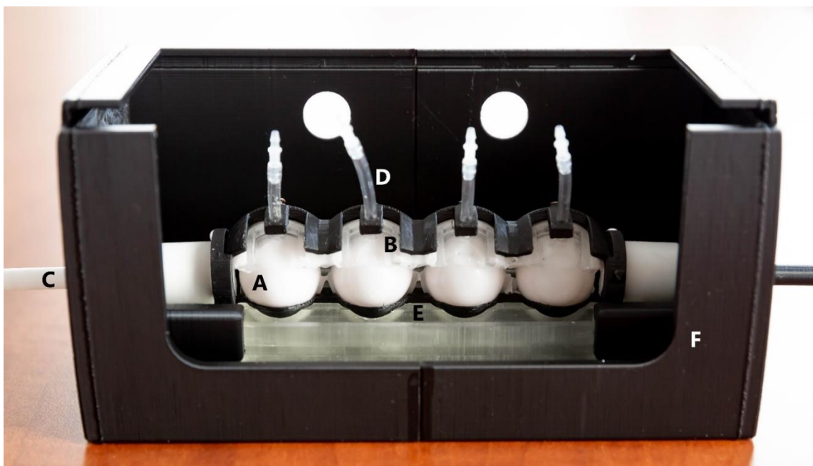
Figure 4.3. OcuBlink 3.0 XL (A) eyeball (B) eyelid in white, with eyelid support structure in black (C) 3D-printed rod to attach to motor (D) tubing to administer tear fluid (E) black 3D-printed lower eyelid with resin support structure (F) 3D-printed chamber.
